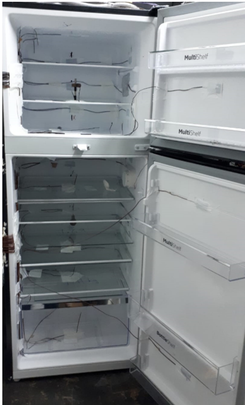
Figure 6.8. Thermocouples placed inside both compartments.
