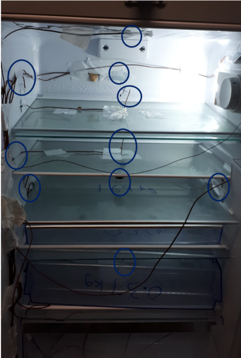
Figure 6.9. Thermocouples (marked with blue circles) inside the FF compartment.
