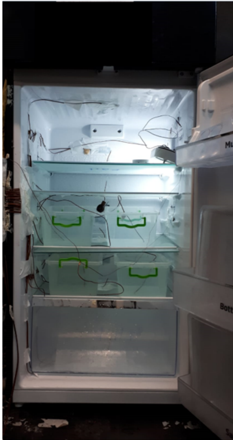
Figure 6.11. FF compartment filled with water pots for the water pot test.
