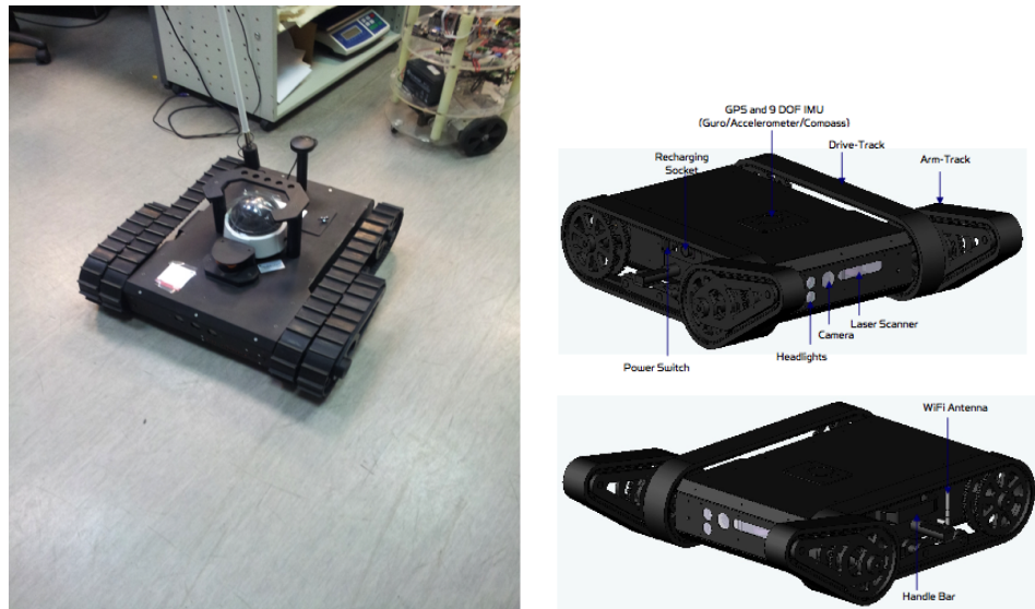
Figure B.1. Left: Jaguar robot; Right: Robot components.
