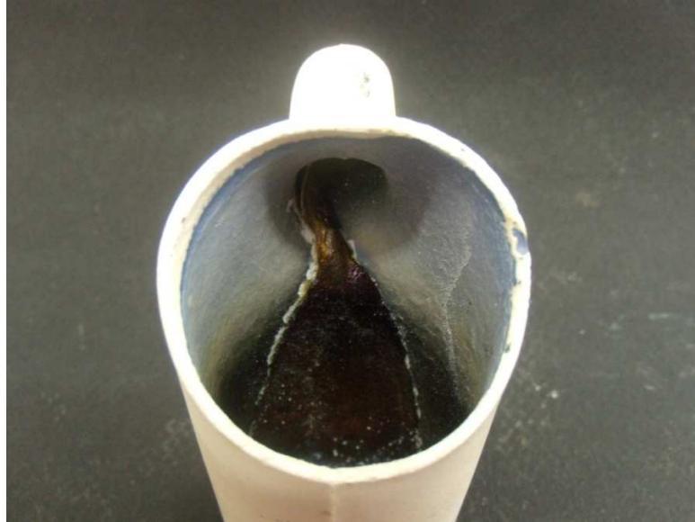
Figure 3.29. The crucible after casting (300/1)
