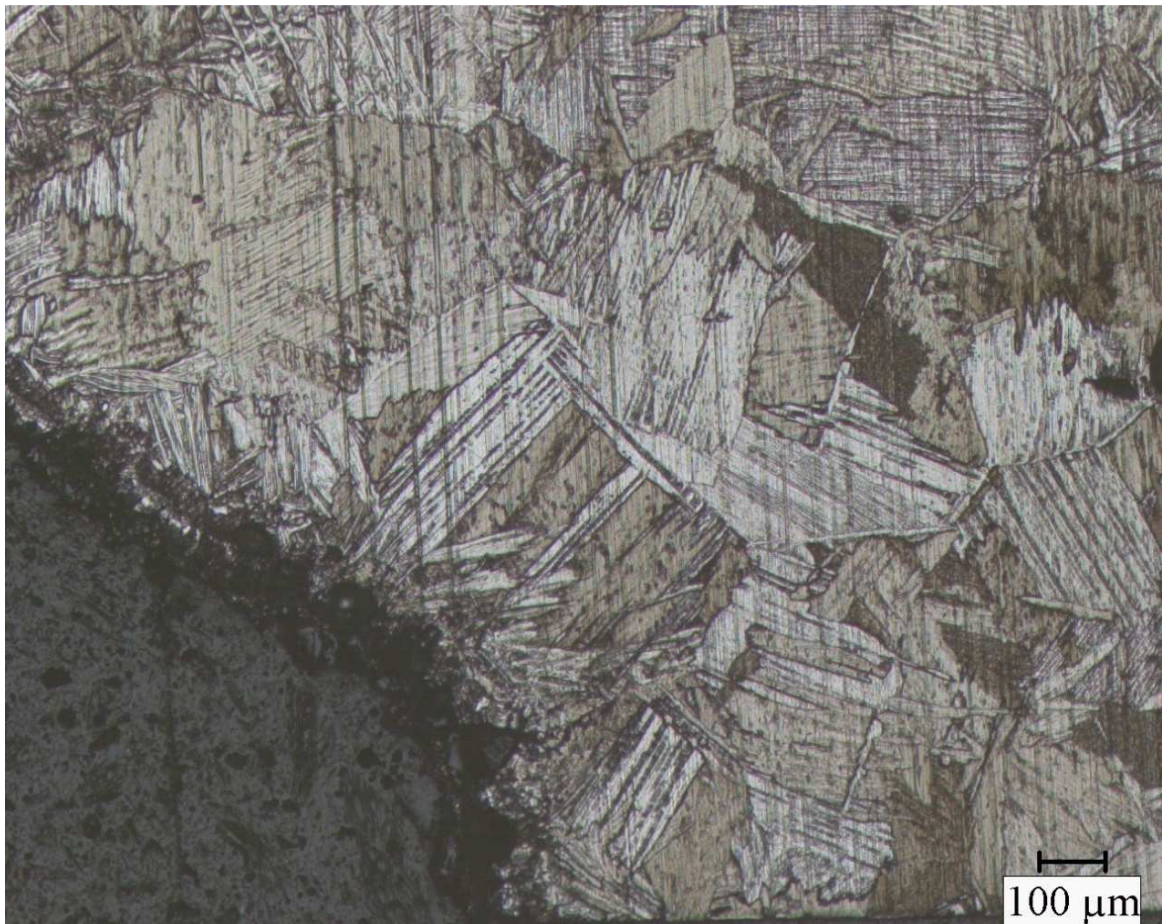
Figure 4.1. Microstructure of 300/1 AC specimen
