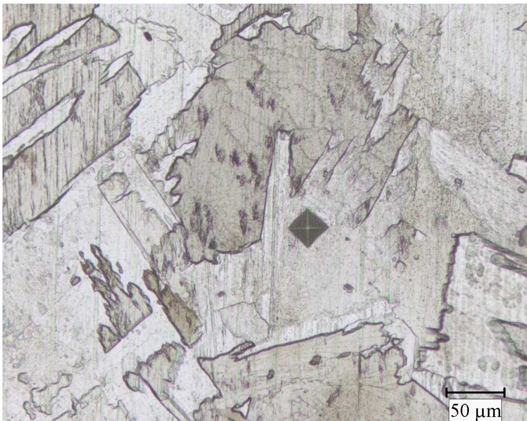
Figure 4.13. Microstructure of indentation in 300/1 AN specimen
