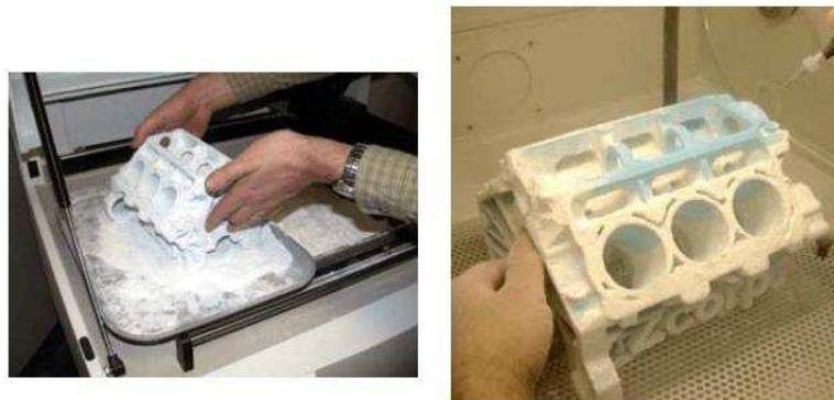
Figure 2.65. Removing the part from the machine and cleaning with compressed air [60]
