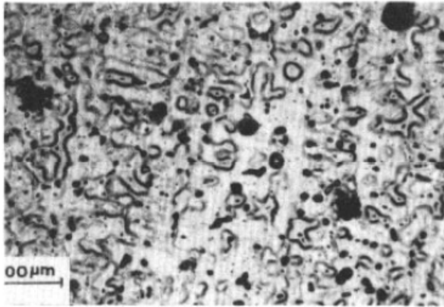
Figure 2.47. Microstructure of centrifuged casting at 1000 RPM [5]
