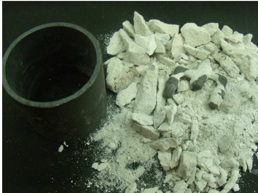
Figure 3.25. An empty muffle after casting, broken investments and the product (300/1)
