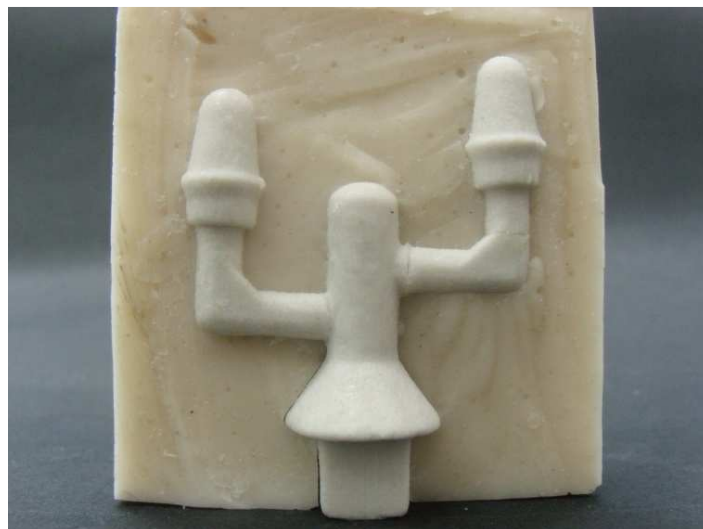
Figure 3.9. Silicone mould and rapid prototyping model
