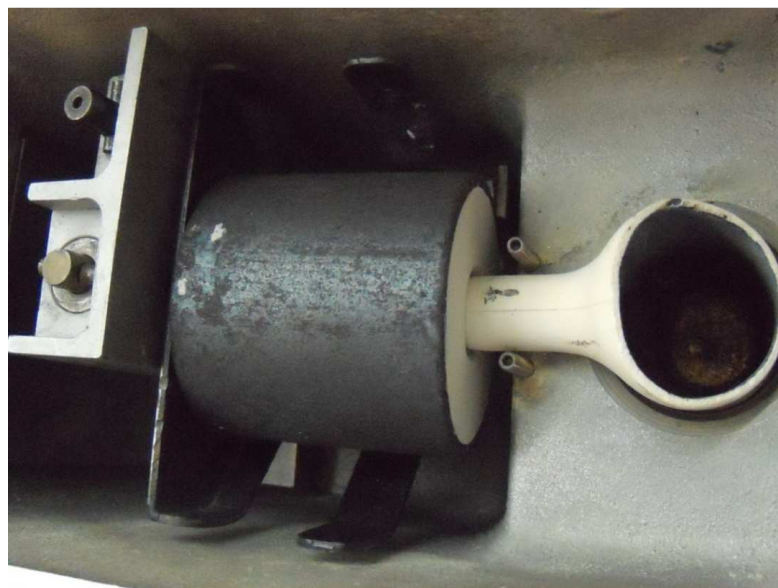
Figure 3.21. Mould and crucible
