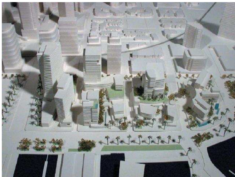
Figure 2.61. A city model printed by ZPrinter 310 Plus [59]
