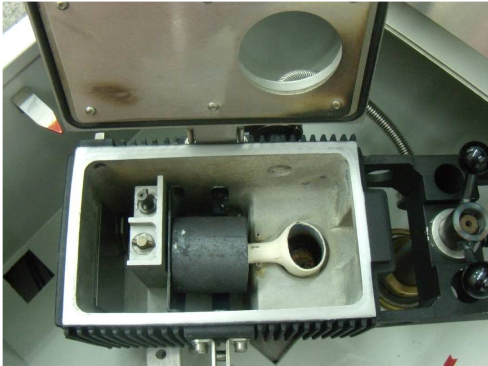
Figure 3.22. Mould and crucible inside the casting arm
