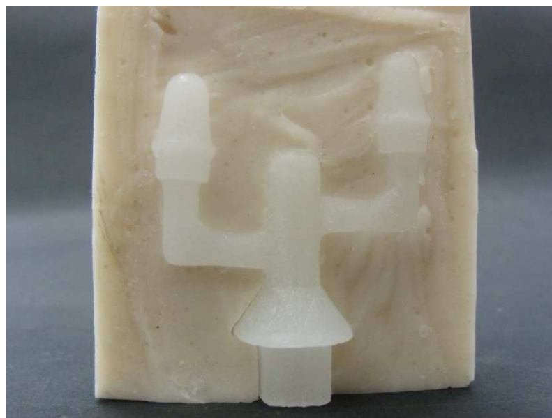
Figure 3.11. Wax model and silicone mould
