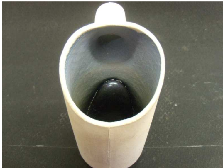
Figure 3.24. Crucible after 200/2 casting condition
