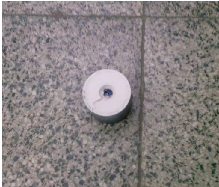
Figure 3.30. 500/1 mould after casting
