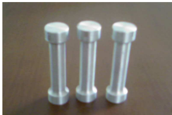
Figure 5.2. Photo of high pressure die casted tensile test specimens
