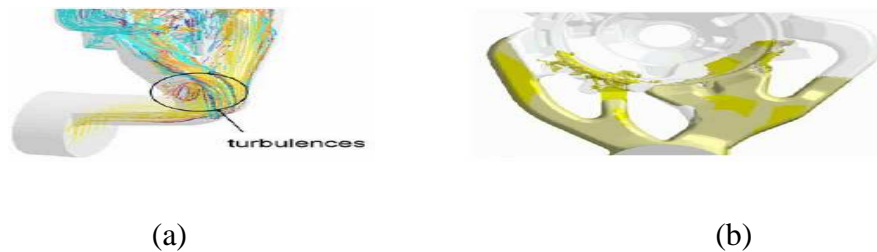
Figure 3.6. (a) Turbulences in the gate due to unfavorable design, (b) Disadvantageous dimensions of the runners lead to uneven die filling. Due to the tight dimensions the right branch of the gate is filled too late [21].
