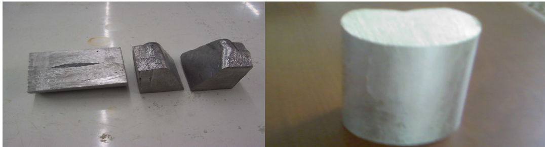
Figure 5.3. Some of the cut Etial 150 pieces before squeeze casting
