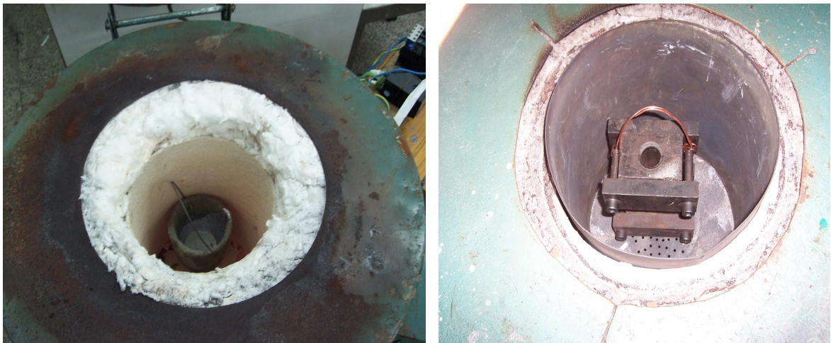
Figure 5.4. The Etial 150 alloy in the pot is moltening in the furnace on the left and the die is being heated in the other furnace on the right.
