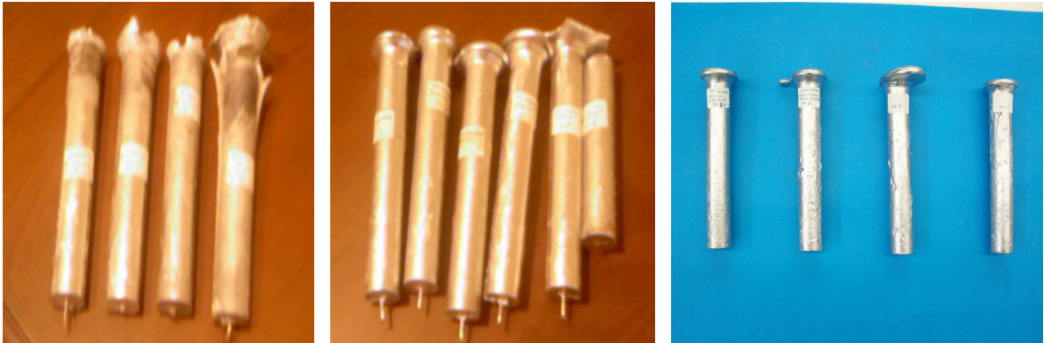
Figure 5.6. Squeeze casted four specimens are seen on the left, six specimens unsqueezed in the hot die are seen in the middle, and four of the six unsqueezed in the cold die specimens are seen on the right.
