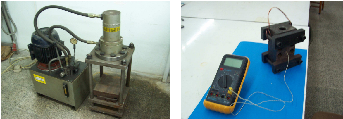
Figure 5.5. Squeeze casting equipment (hidrolic press) is on the left and the die with micrometer in order to measure the temperature is on the right
