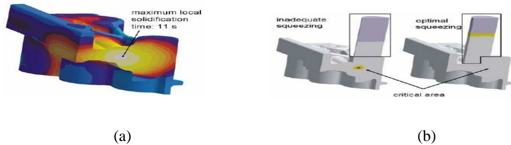
Figure 3.16. (a).The maximum solidification time occurs in a thick-wall area of the casting. (b).Depending on the design of the squeezing system, shrinkage cavities can be avoided at the critical area (right) [19].
