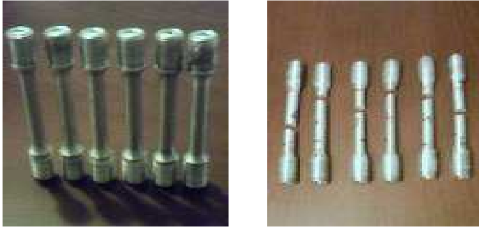
Figure 5.16. Six tensile testing specimens of unsqueezed in the cold die casting; before tensile testing on the left and after tensile testing on the right photo
