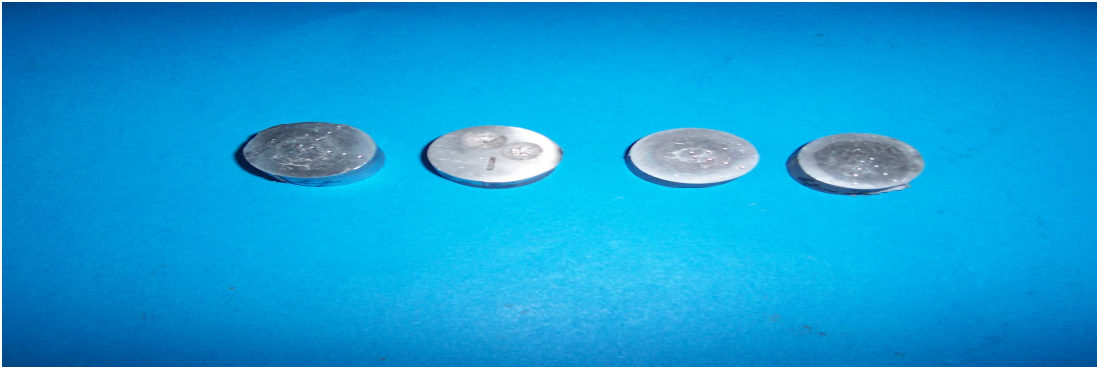
Figure 5.10. Photo of hardness specimens of squeeze castings
