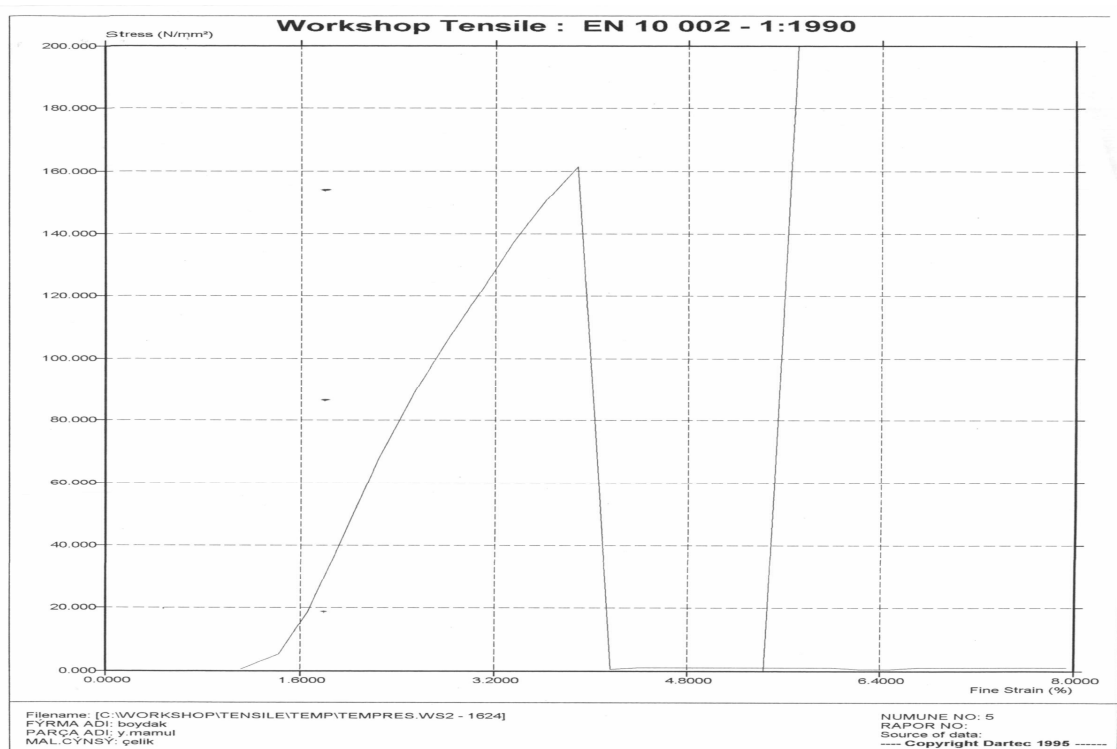
Figure A.8. Stress-strain curve of the fifth not-squeezed sample
