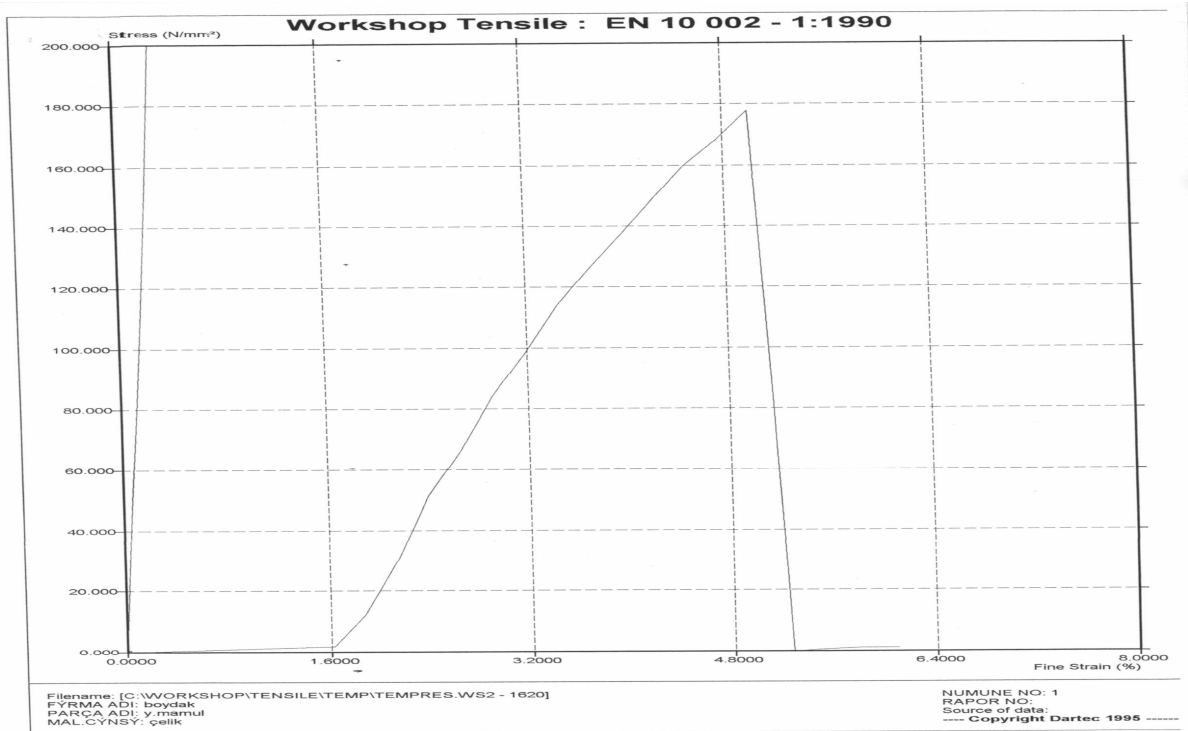
Figure A.4. Stress-strain curve of the first not-squeezed sample
