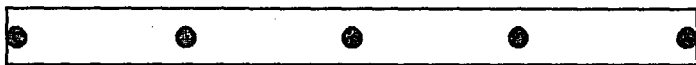
Fig.3.1. Lumped parameter model of the flexible shaft. The shaft is divided in to n_s segments. Mass of each segment is equally divided in to each end.
