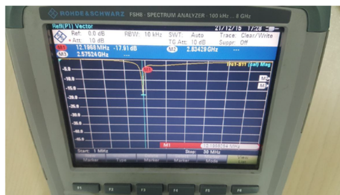
Figure 4.18. Shifted operating frequency with the effect of metal (2cm distance).
