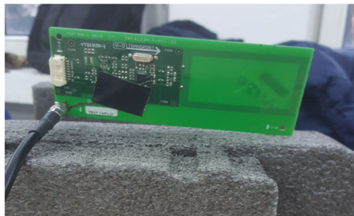
Figure 4.15. Experimental setup of reader with rectangular antenna.
