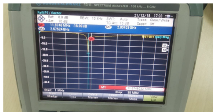
Figure 4.16. Spectrum Analyser measurement of reader with rectangular antenna.
