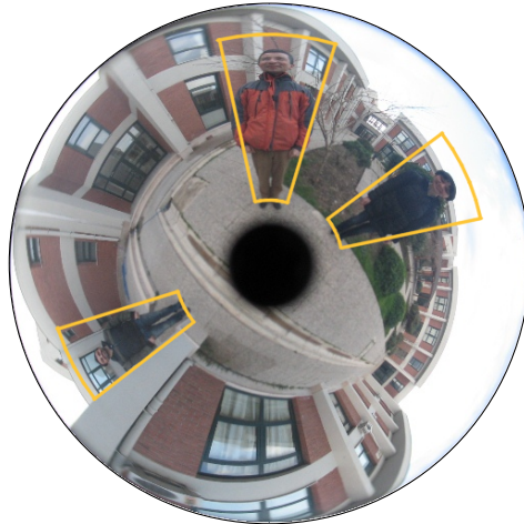
Figure 3.1. Person detection in an omnidirectional camera setting, with the detection results of the proposed approach superimposed.
