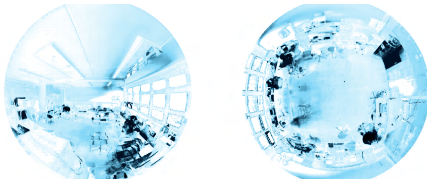
Figure 2.2. Illustration of the standard deviation of image pixel intensities for the V channel of HSV color space. Darker colors indicate higher deviation.
