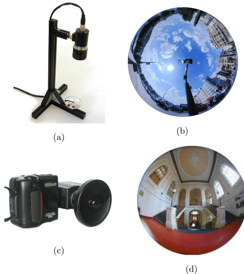
Figure 1.1. Examples of catadioptric and dioptic systems and acquired images using those cameras [20]. (a) Catadioptric system with a hyperbolic mirror. (b) Image acquired with a catadioptric system. (c) A camera with a fisheye lens. (d) Image acquired with a fisheye camera.
