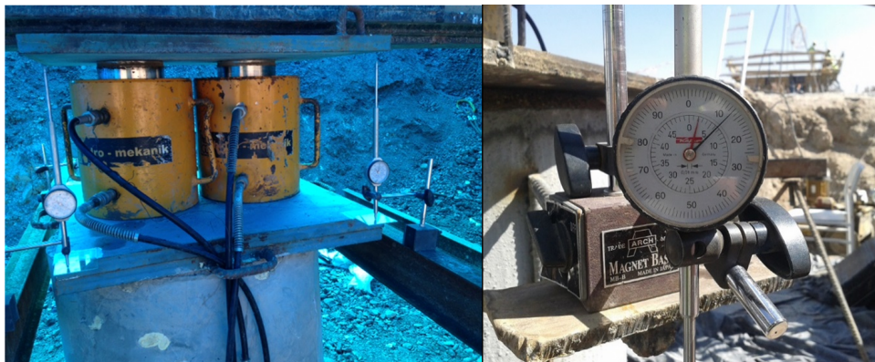
Figure 4.4. Measurement of movements.
