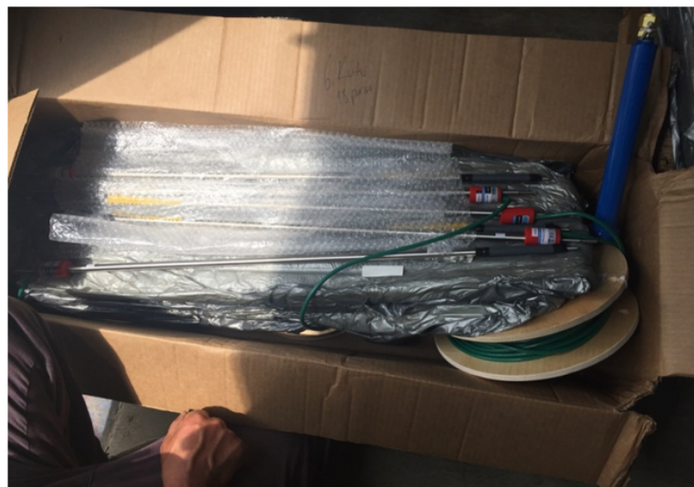
Figure 5.4. Linear vibrating wire displacement transducers (LVWDT).
