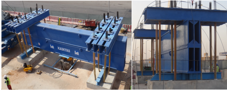
Figure 4.3. Test arrangement by using ground anchors.
