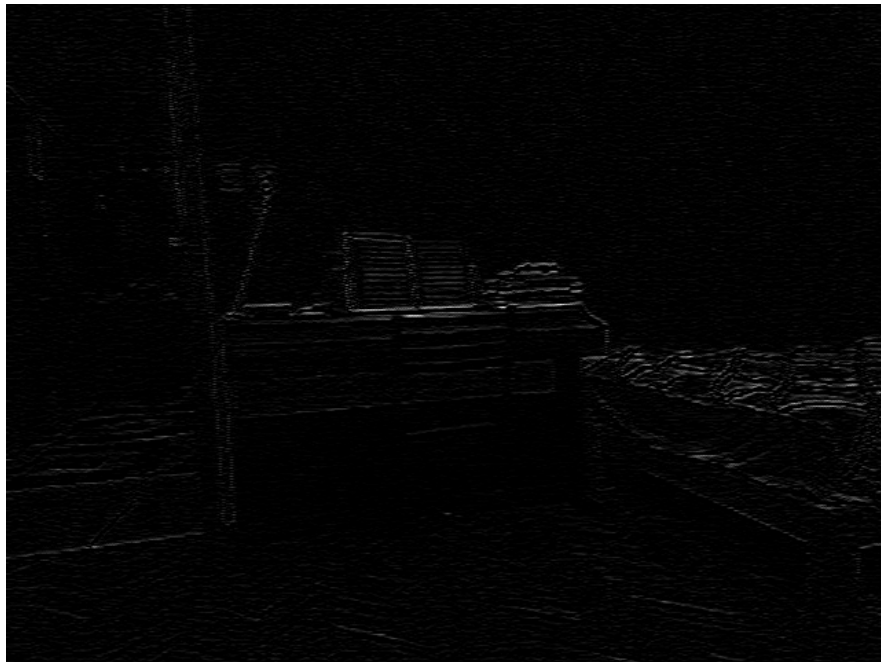
Figure 2.7. Resulting activation map of applying horizontal line filter (filter A) to the image in Figure 2.6.
