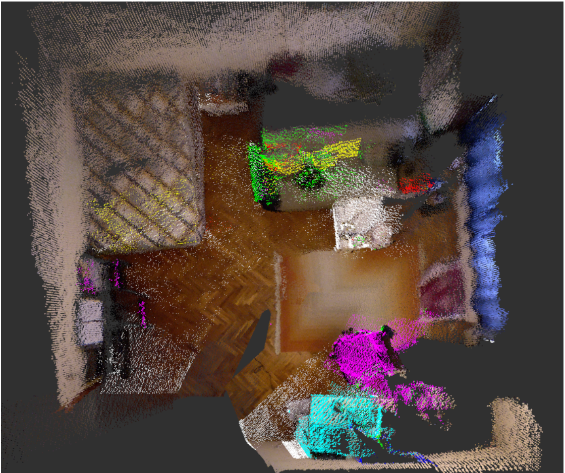
Figure A.7. 3D semantic maps of the first room using the SSD-RGB and SSD-D+ fusion as the object detector.
