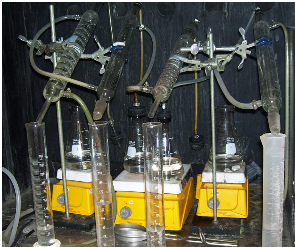
Figure 4.5. Distillation setup for VFA analysis
