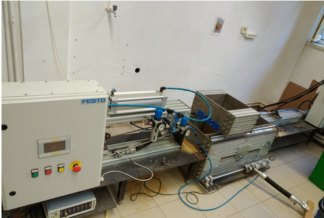
Figure 4.2. Overall view of large-scale direct shear device.
