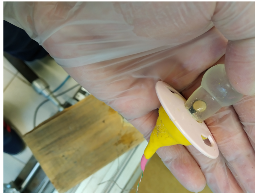
Figure 4.1. The miniature stress transducer enclosed in pacifier.
