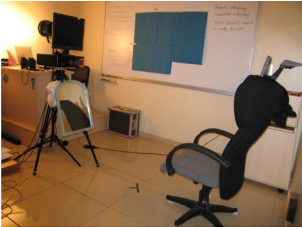
Figure 3.2. Acquisition setup composed of a 3D digitizer, a mirror, an LCD display, a 1000W halogen lamp, a seat (1.5m away from the digitizer), and yellow straps to indicate rotation angles (on the floor, just below the seat).
