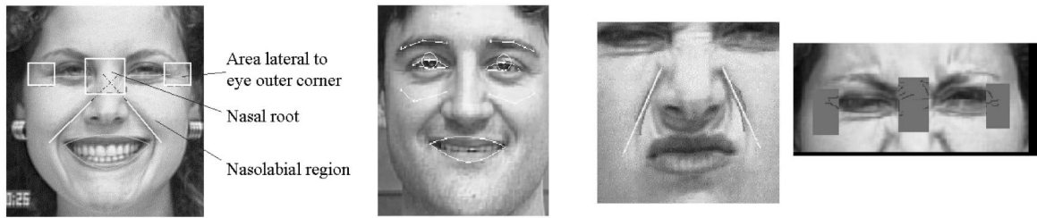
Figure 2.4. Facial feature extraction by Tian et al. [33]. Permanent and transient facial features like nasolabial furrows are extracted by geometric model fitting.
