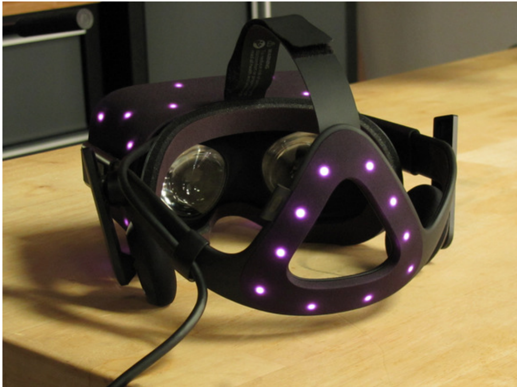
Figure 5.1. Oculus Rift Consumer Version infrared markers.
