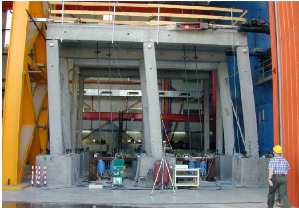
Figure 4.3. The picture of the deformed precast building, Ferrera and Negro (2004)
