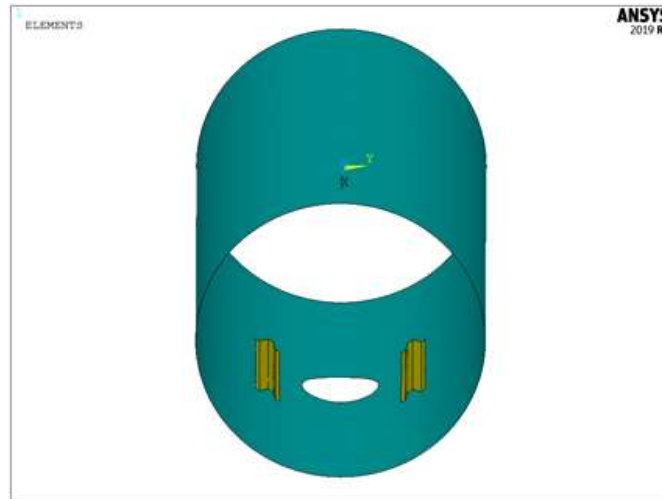
Figure 4.13. B100 cylinder with stiffeners applied.
