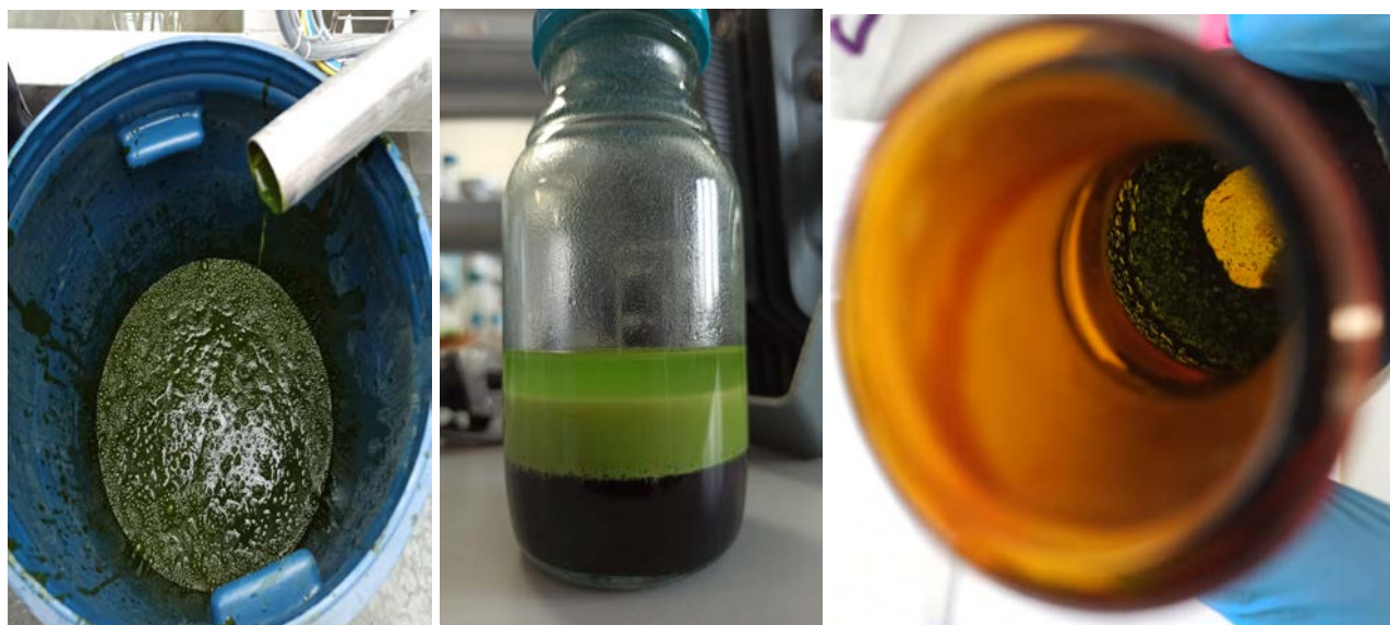
Figure 3.11. Homogenized N. gaditana in barrel (left), chloroform:methanol phase separation stage during lipid extraction (middle), lipid extracts after chloroform evaporation (right).
