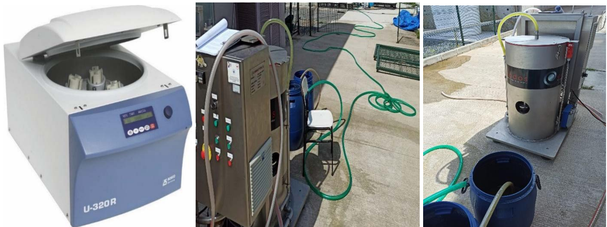
Figure 3.7. Centrifuge and decanter Evodos T10 used for harvesting and dewatering.
