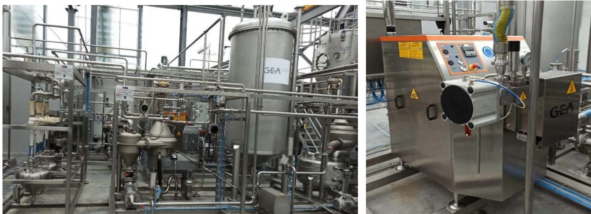
Figure 3.8. Hydrocyclone, separators (left) and homogenizer (right) for large-scale dewatering.
