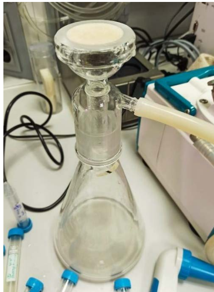
Figure 3.9. Filtering unit for dry weight measurements.
