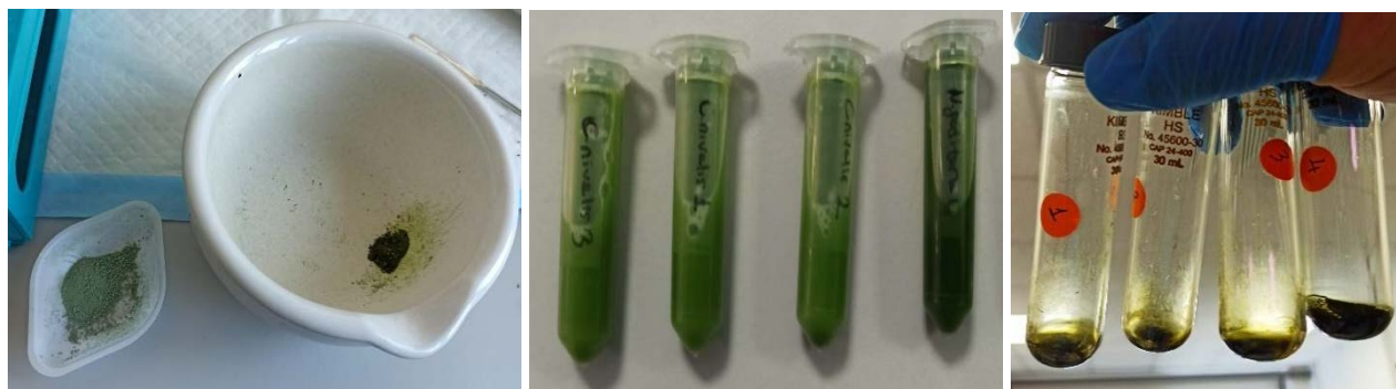
Figure 3.10. Lyophilized microalgae powder (left), dried microalgae in chloroform:methanol solution in bead milling tube (middle), algal lipid extract samples (right).
