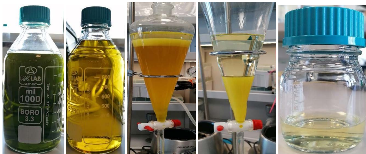
Figure 4.42. From left to right: crude extract before and after chlorophyll removal, chloroform extraction of crude extract, n-hexane extraction of crude extract and esterified algal lipids.
