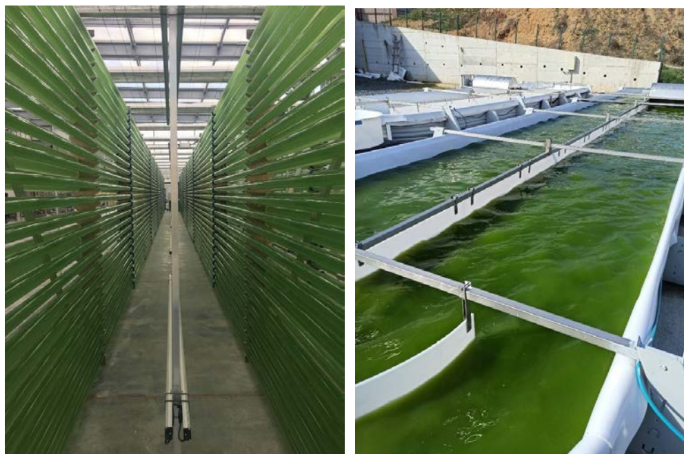
Figure 2.5. Closed tubular PBRs (left) and open raceway pond (right) available at IMBIYOTAB facilities.
