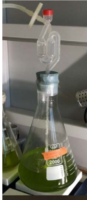
Figure 3.2. Small-scale PBR design in 2L Erlenmeyer flask.
