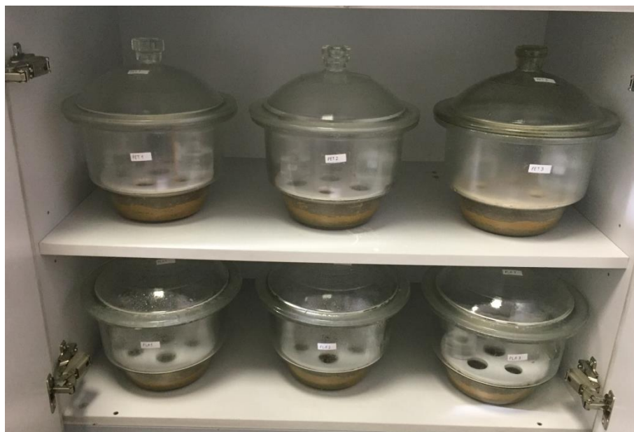
Figure 3.7. Sealed reactors placed in a dark cabinet.
