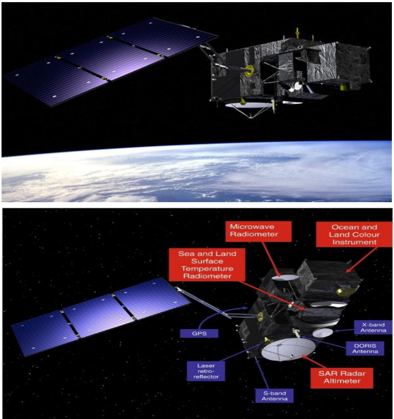
Figure 5.7. Sentinel-3 Satellite and payloads (ESA).
