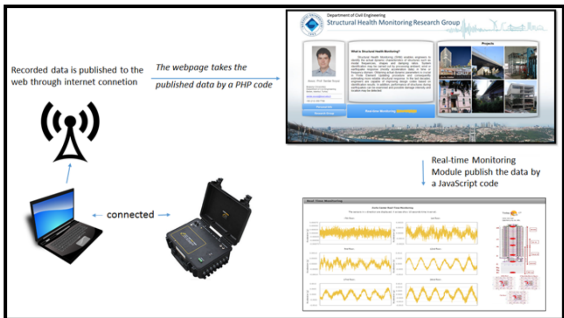
Figure 3.5. The steps of “real-time monitoring” module.
