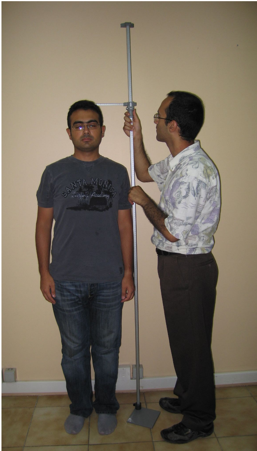
Figure 4.6. Measurement of height with the anthropometer
