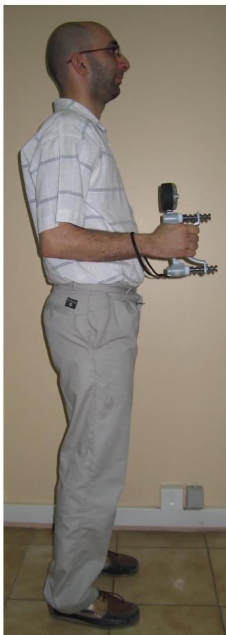
Figure 4.10. Measurement of grip strength value of right hand while the subject is standing and dynamometer is unsupported
