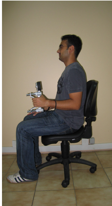
Figure 4.12. Measurement of grip strength value of left hand while the subject is sitting and dynamometer is unsupported
