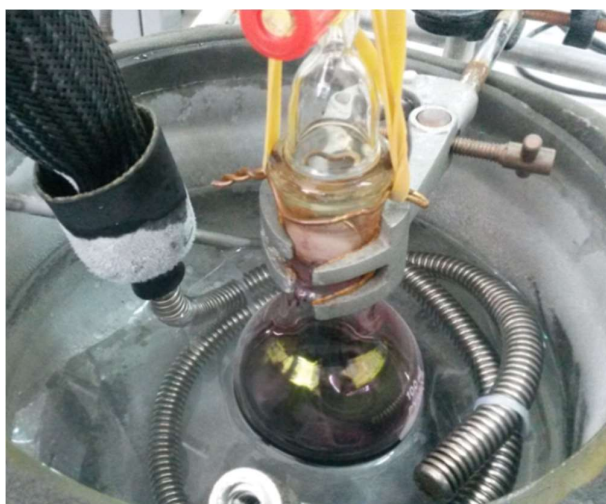
Figure 3.2. Synthesis of anthryl telechelic poly(methyl methacrylate) by anionic polymerization.
