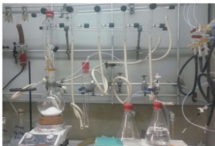
Figure 3.4. Synthesis of 5-tert-butyl-1,3-bis(2-chloro-2-propyl)benzene.
