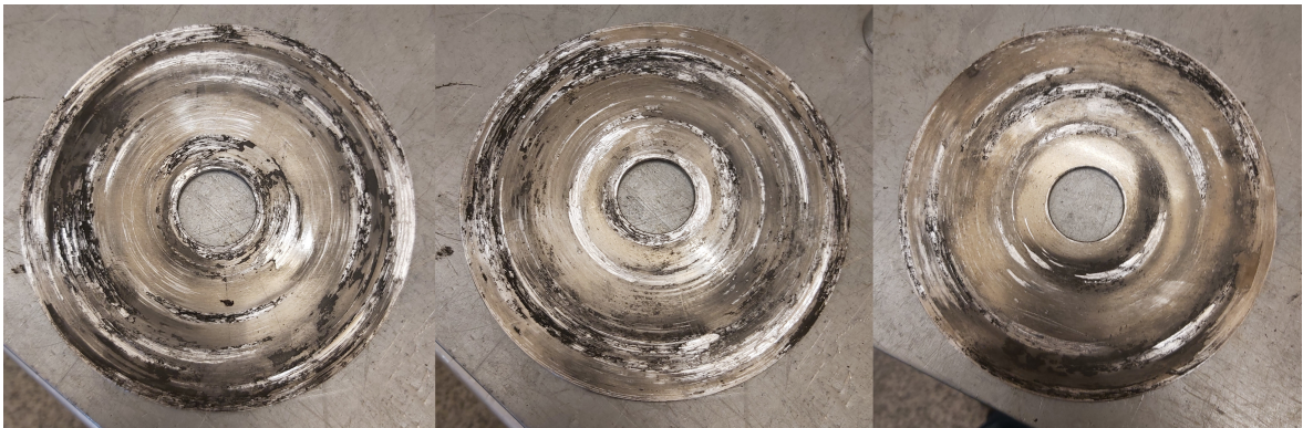
Figure 2.28. Aluminum alloy friction disks after the experiment.
