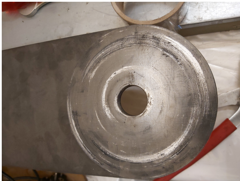
Figure 2.30. Damper plate friction surface experiment.
