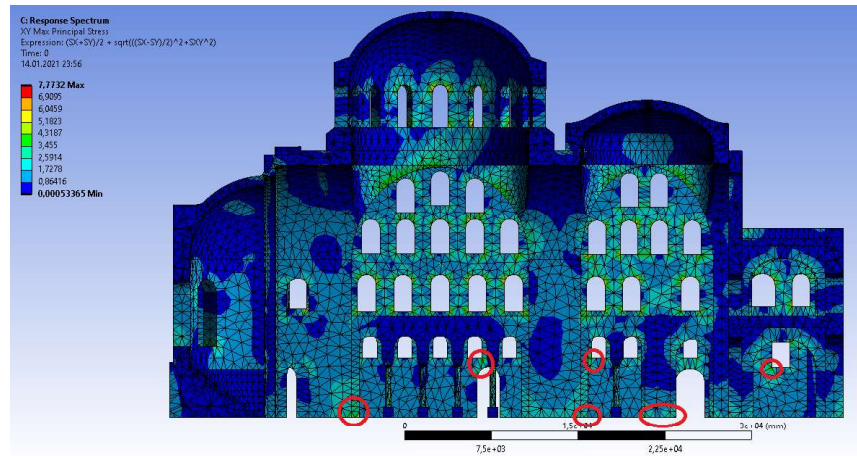
Figure 7.7. Entry 1 Damages FEM Results
