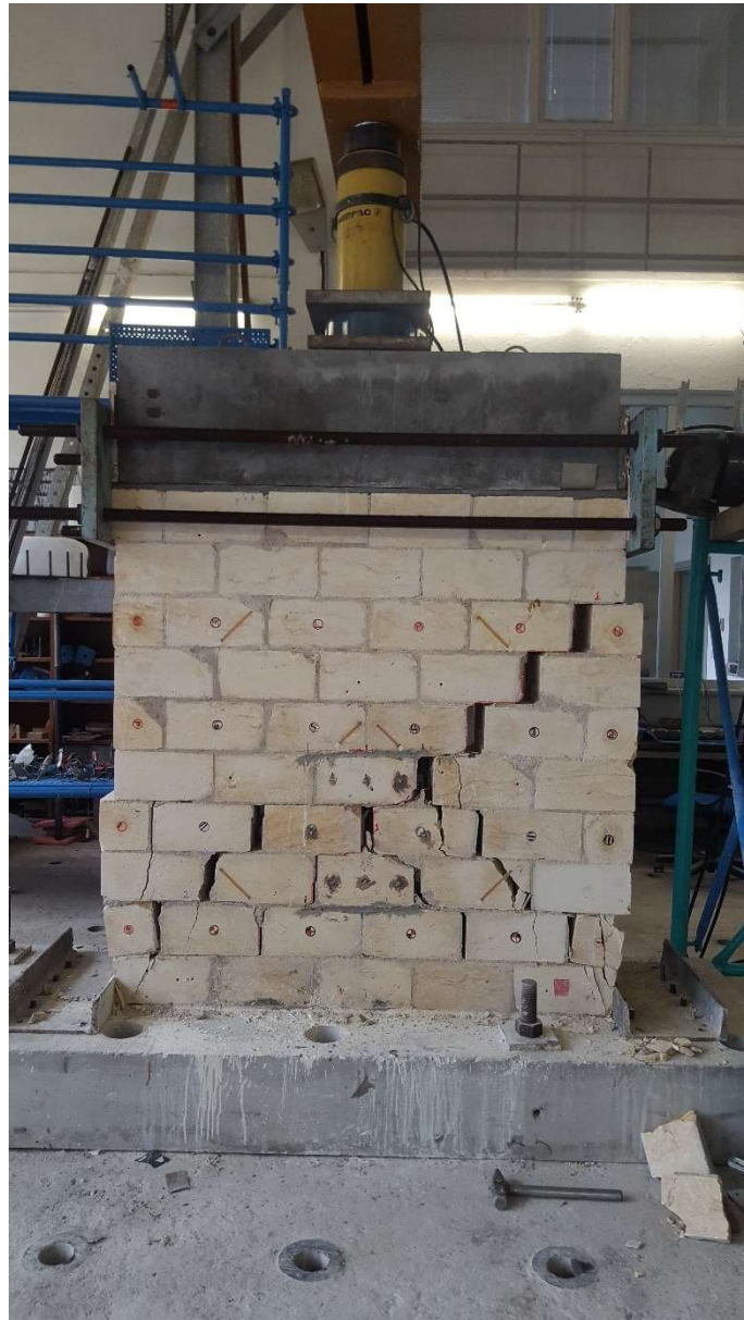
Figure 4.6. Damaged Wall After The Test
