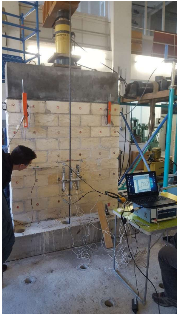
Figure 4.2. Masonry Wall During Flat Jack Test
