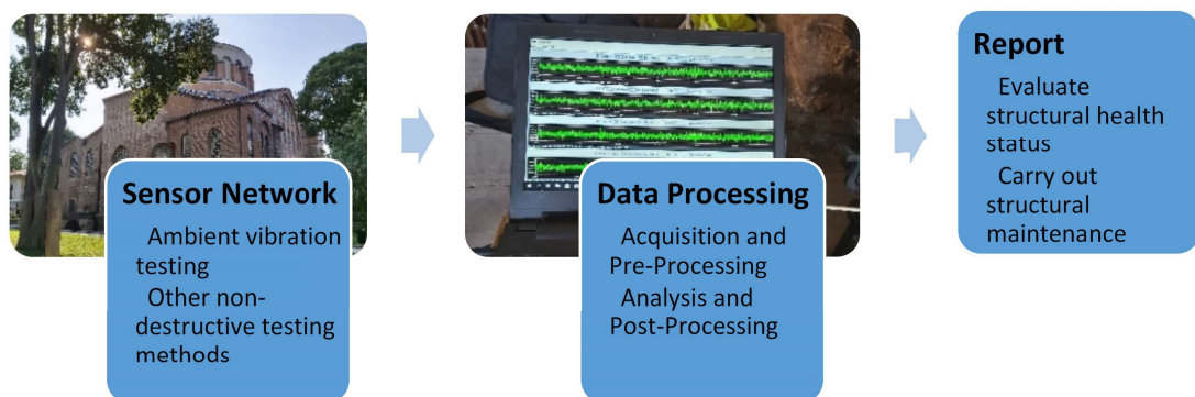
Figure 2.1. Typical Structural Health Monitoring System
