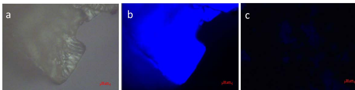
Figure 4.19. Optical fluorescence microscopy image of (a), functionalized hydrogel (bright field), (b) upon excitation at 365 nm, and (c) control experiment upon excitation at 365 nm.
