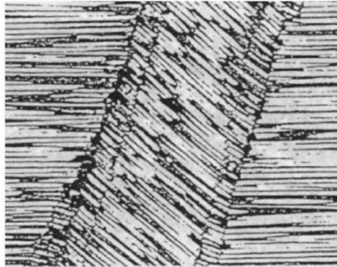
Figure 2.17. Micrograph of a unidirectional composite kink-band [48].
