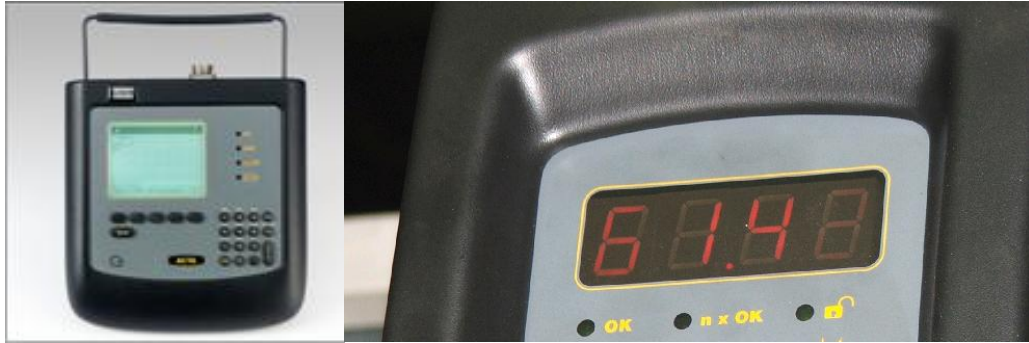
Figure 4.5 Bolt torque measurement equipment - ACTA 3000
