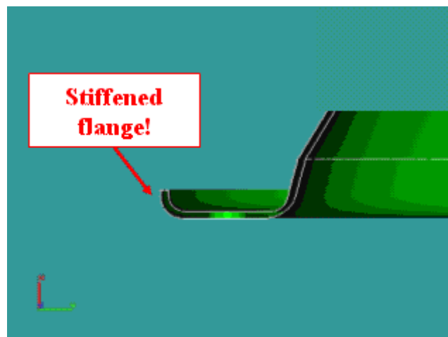
Figure 2.2. Proposed cover (Cover 2&3) flange design
