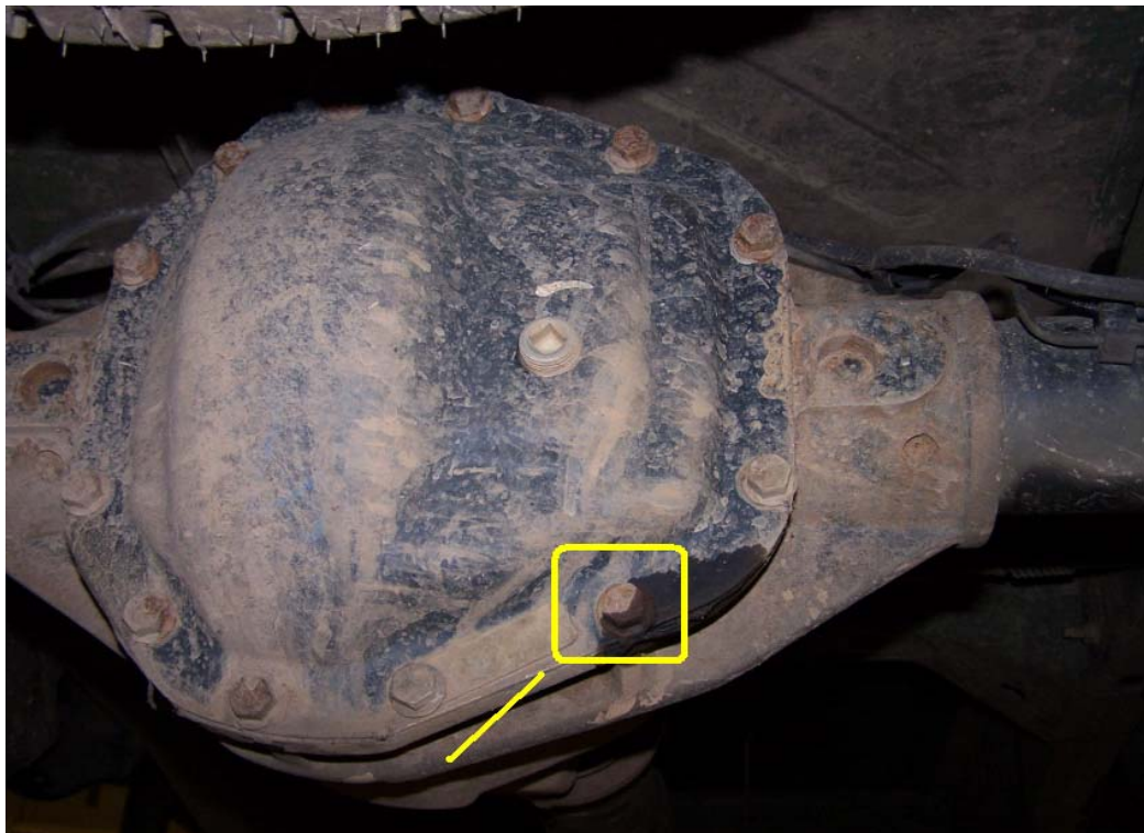
Figure 2.7. Leakage from rear axle cover 1, after TTGD test
