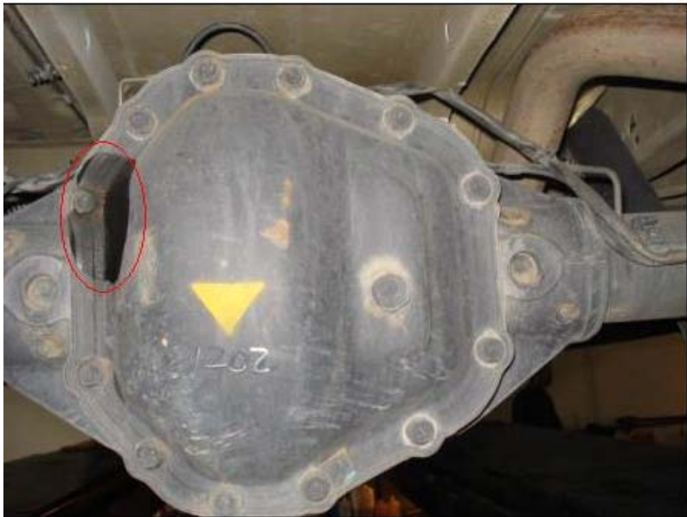
Figure 2.9. Leakage from rear axle cover 2 after TTGD test
