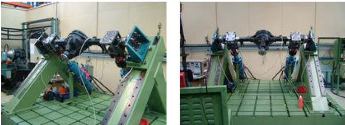
Figure B.1. Rear axle beam fatigue test rig
