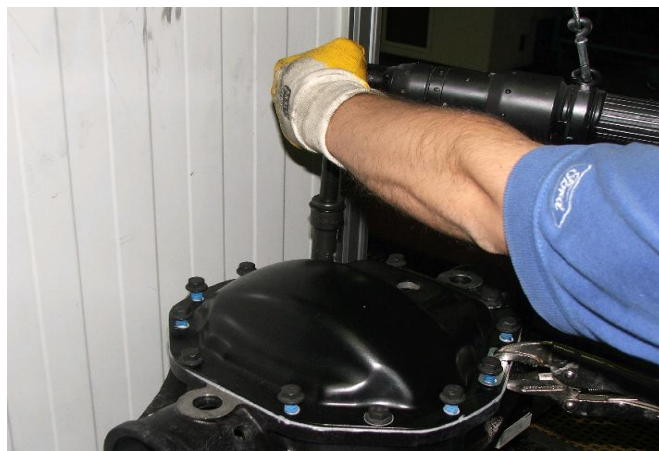
Figure 4.4 Bolt tightening process and torque equipment
