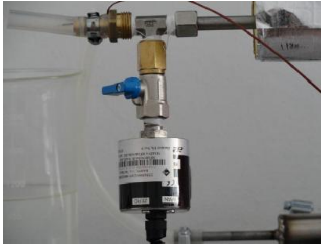
Figure 2.4. Pressure transducer connected to the test setup.
