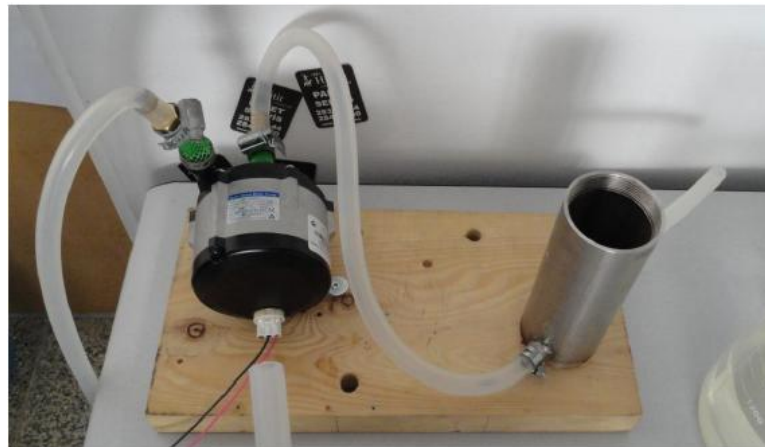
Figure 2.5. The pump and the reservoir.
