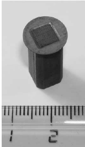
Figure 2.3. Photograph of Rh-impregnated microchannel reactor [22].
