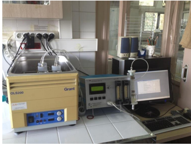
Figure 3.3. Configuration of respirometry tests
