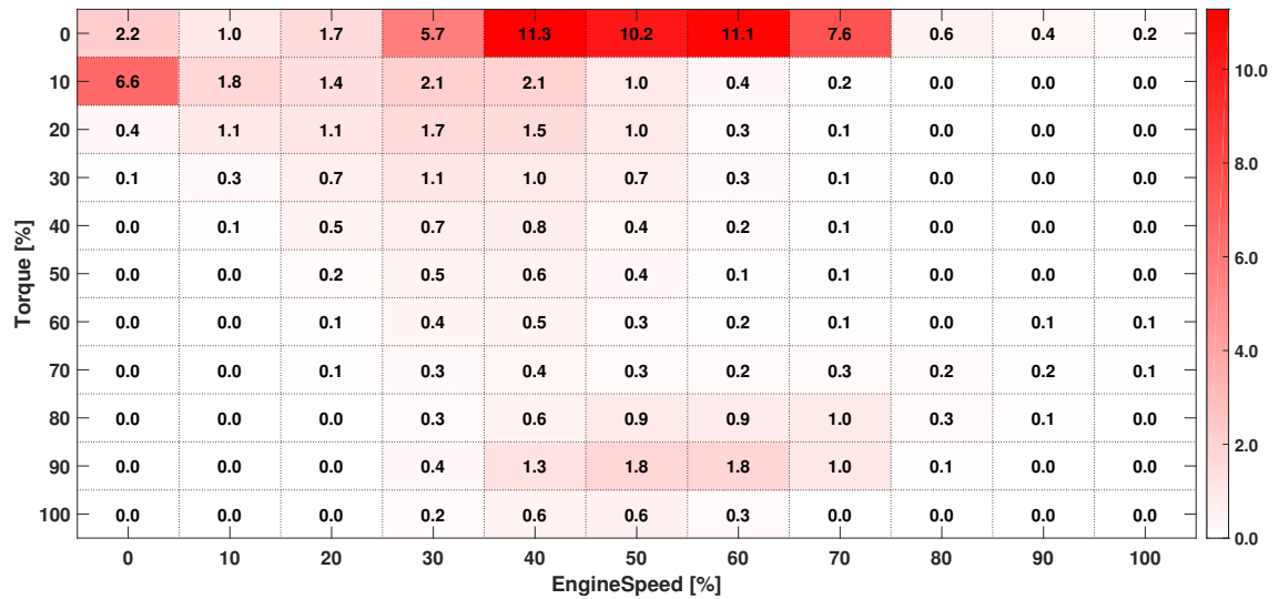
Figure 3.9: Distribution of time spent on a normalized engine speed - torque map. The color of a point is getting darker as the frequency increases.
