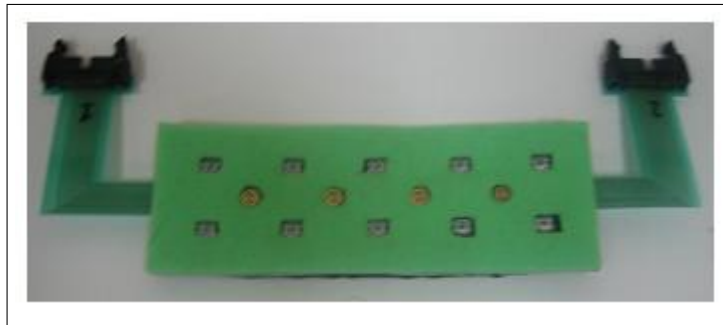
Figure 3.2 A 4-LED probe with 10 photodetectors
