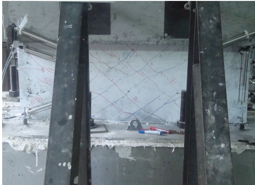
Figure 3.17. Diagonal Cracking Pattern at Ultimate Load Level (T4-S1).
