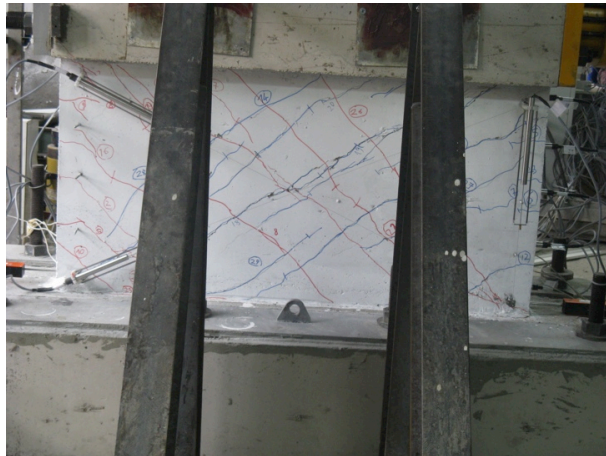
Figure 3.2. Cracking Pattern at Ultimate Load (T1-S1).
