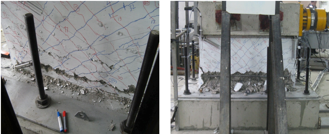
Figure 3.6. Medium and High Damage Levels (T2-S1).
