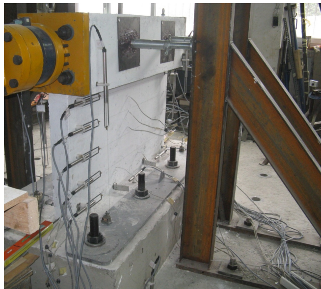
Figure 2.35. Vertical and Horizontal LVDTs.
