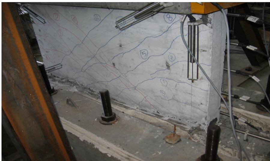
Figure 3.11. Cracking Pattern at Ultimate Load Level (T2-S3).
