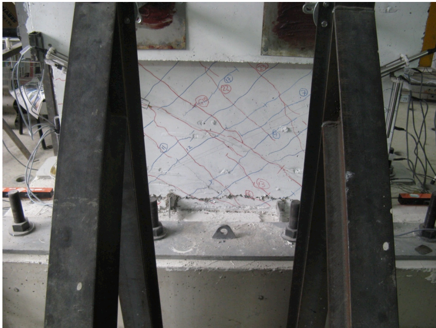
Figure 3.8. Cracking Pattern at Ultimate Load (T2-S2).
