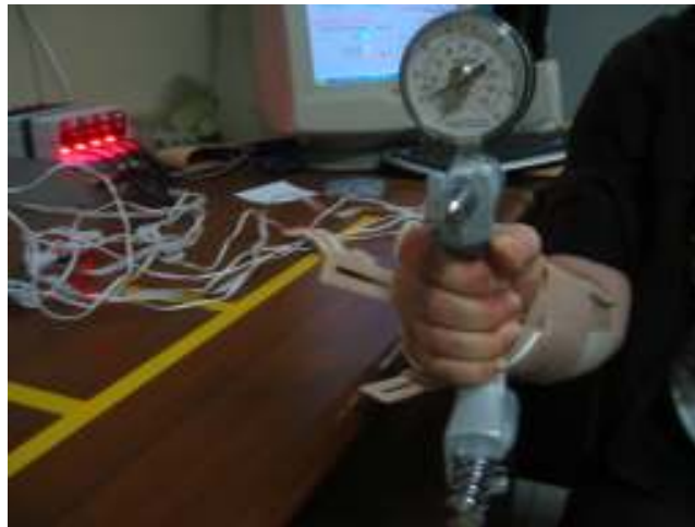
Figure 3.41 The implementation of the grip strength measurement test with the NeO
