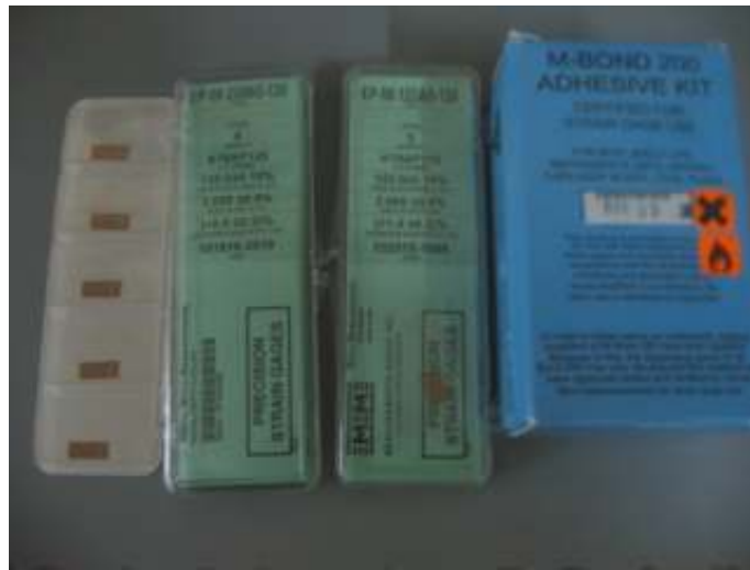
Figure 3.2 Strain gauges and the adhesive used in the experiments
