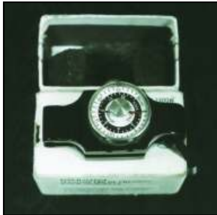
Figure 3.36 B&L Pinch Gauge
