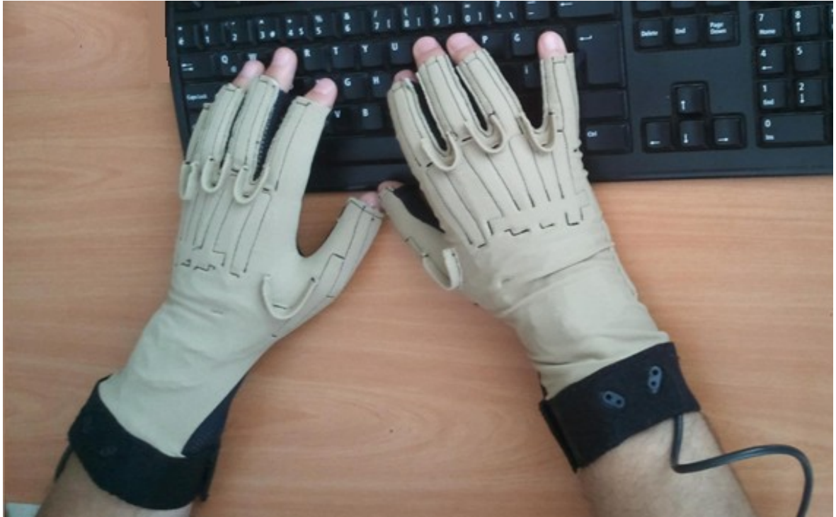
Figure 6.9. The edges of the fingers were cut to allow the subjects to feel and touch the keys and in female subjects latex examination gloves were worn in order to prevent sliding during the typing
