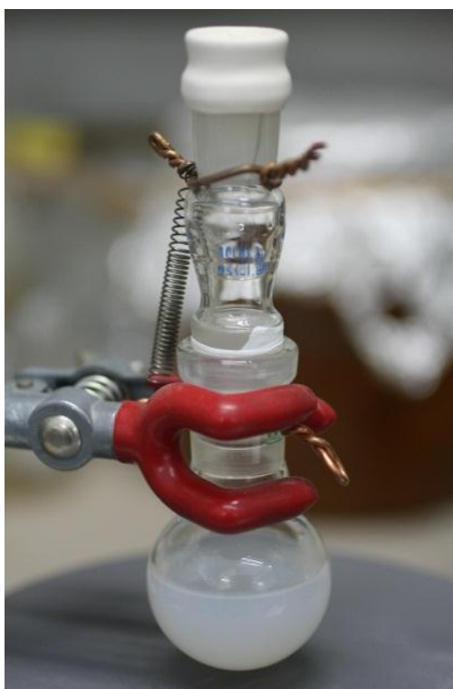
Figure 3.4. Reactor setup for hydrolysis with amine usage
