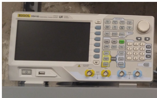
Figure 3.11. The signal generator selected for providing the input signal: RIGOL-DG4102.
