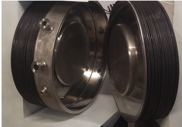
Figure 3.8. Vacuum chamber of OZU Cyclotron
