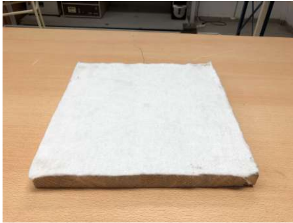
Figure 3.8. 300mm-300mm Geotextile for Interface Experiments.
