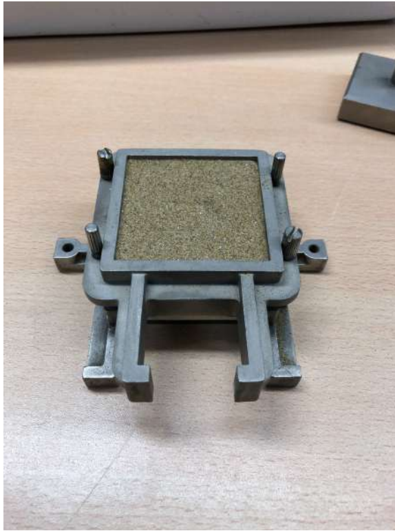
Figure 3.2. Shear Box 60mm-60mm.
