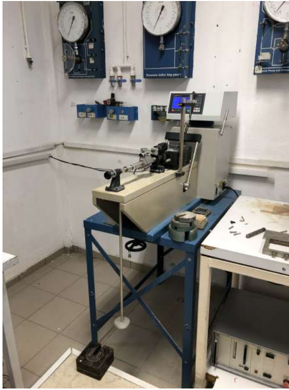
Figure 3.1. Traditional Direct Shear Device.
