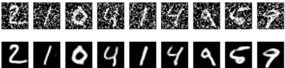
Figure 4.3. The row above contains 9 randomly selected noisy test samples and the row below contains the autoencoder model's denoised output [64].
