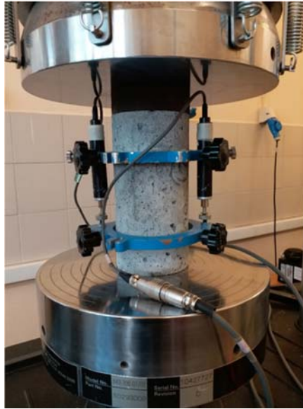
Figure 2.5. Elastic modulus test setup
