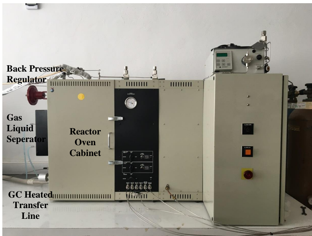
Figure 3.3. The Autoclave Engineer's BTRS-Jr-PC high-pressure fixed bed reactor system.
