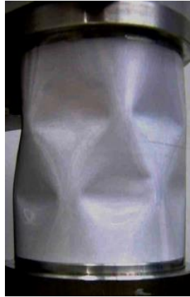
Figure 2.7. Buckled shell under axial compression [20].
