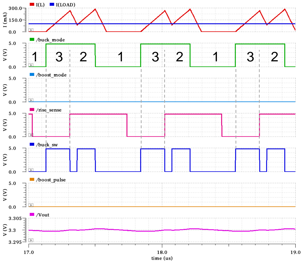
Figure 5.5. Simulation results for V_{IN}=4.8V , V_{OUT}=3.3V I_{LOAD}=100mA .
